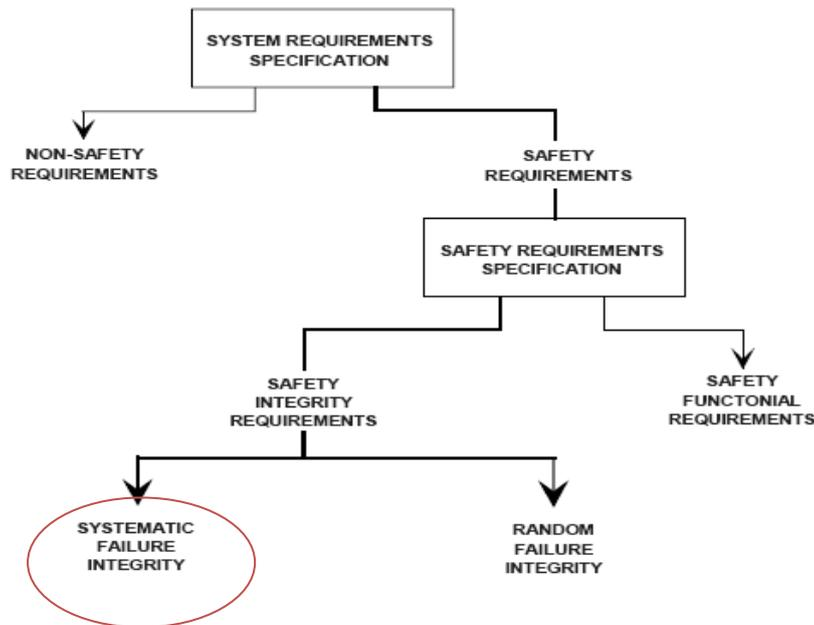
Figure 2 Systematic Failure Within a System
